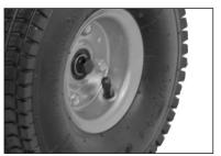
2. Wheel split pins fitting.Fit with split pins just tight enough to get split pins in.
